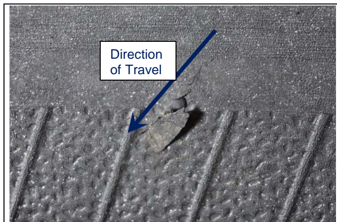
Figure 2. Gouge in Inner Liner under tread at the 9:10 clock position.
