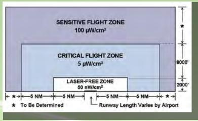
Figure 1: Protected Flight Zones for a Single-Runway Airport
