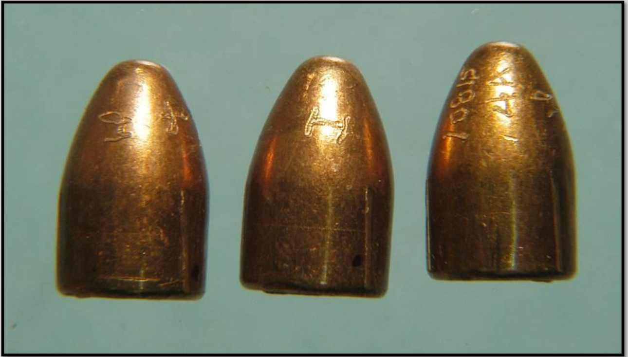
3 "INDEPENDENCE" 115gr. 9mm FMJ DPS TEST-FIRED BULLETS Engraved 4A, 4B and 4C on their ogives
